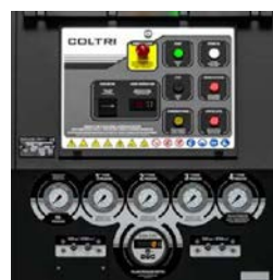
Digital pressure gauges, interstage control + entry pressure
